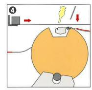
The screen frame starts moving back. The flo-coater starts moving down onto the screen when the squeegee lifts up.
