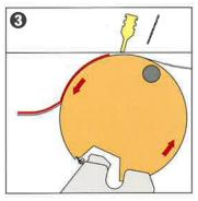
The substrate is delivered after being released by the grippers. The cylinder continues to rotate after the substrate is delivered.
