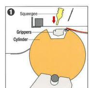
The grippers hold a substrate at the right position while the cylinder stops. Then the squeegee moves down onto the screen.
