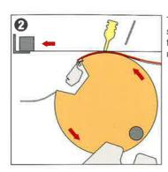
The squeegee moves down and printing starts at the top of the cylinder. The screen frame moves and the vacuum cylinder rotates
