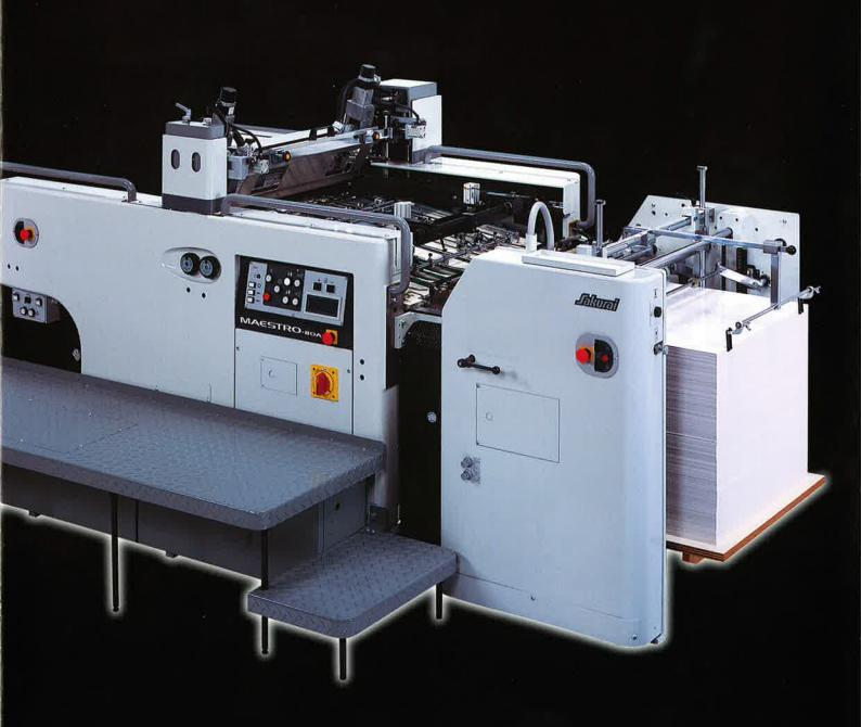
The combination of high precision and productivity - Fully Automatic Ultra-High Precision Rotary, Stop Cylinder Screen Press
