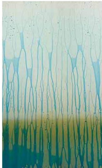
Untreated high-modulus fabric: nonuniform wetting
