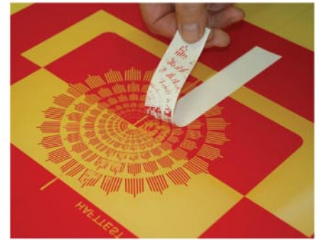
Mesh without surface treatment: part of the emulsion are remaining on the tape
