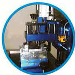
▲ Pneumatic Squeegee Stand / Moving Up and Down
